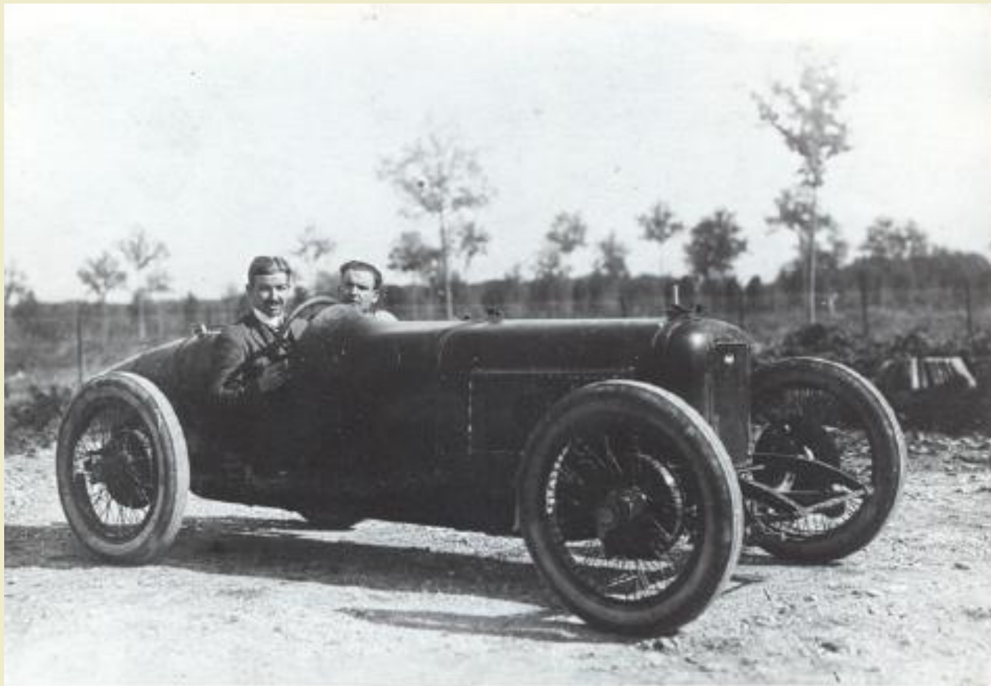
Maserati's brothers in the supercharged 8-cylinder Diatto Gran Prix, the forerunner to the Maserati Type 26
